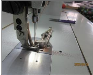
External photo(s) of the production unit(s) Finding 7.17 no needle guard for the sewing machine.JPG
