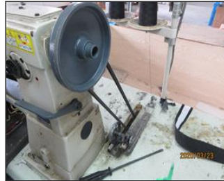
External photo(s) of the production unit(s) Finding 7.17 no pulley guard for the sewing machine.JPG
