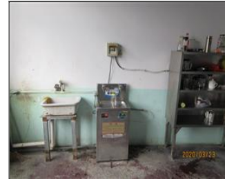
External photo(s) of the production unit(s) Finding 7.9 no warning sign for high temperature.JPG
