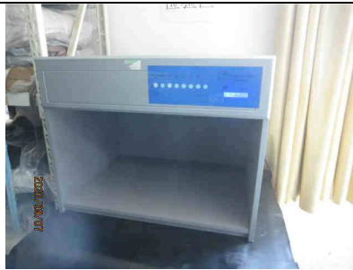
17) light box was not affixed with calibration sticker at incoming materials inspection area
