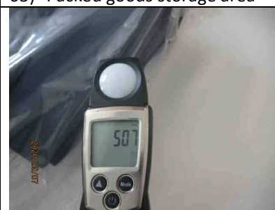
66) Insufficient lighting at final QC area (507 Lux)
