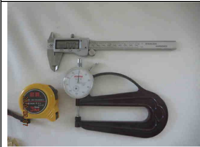
16) Tape measure, caliper and thickness tester were not affixed with calibration stickers at incoming materials inspection area
