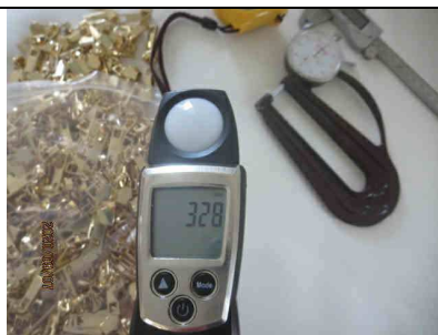
14) Insufficient lighting at incoming materials inspection area (328 Lux)
