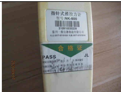
68) Valid calibration sticker was affixed on pull tester
