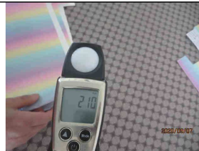
36) Insufficient lighting at in-line inspection area of gluing workshop (210 Lux)
