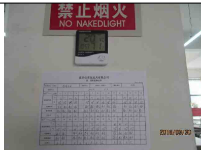
13) Temperature and humidity gauge equipped
