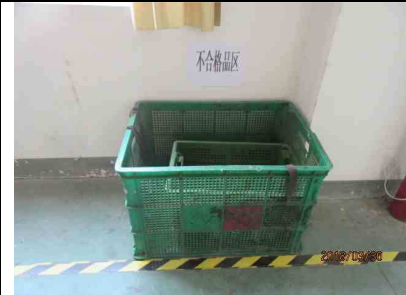
72) Designated nonconforming products storage area
