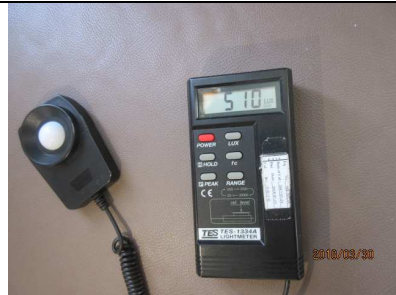
16) Insufficient lighting at incoming inspection area (510 lux)
