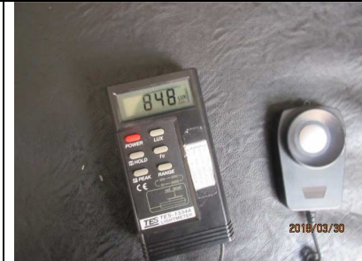
71) Insufficient lighting at final inspection area (848 lux)
